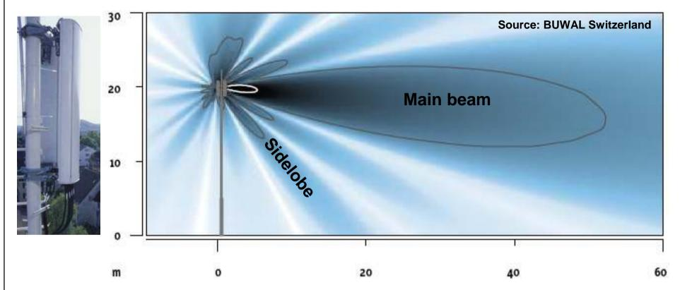
Radiation of a 20 m tall sector antenna for mobile communication (GSM 900 MHz) with an effective radiated power (ERP) of 1000 Watt (Distances in Meters)
